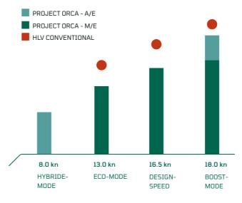
"Compared to conventional heavy lift vessels, fuel consumption is 45% lower in eco mode (13kn) and approx. 33% lower in cruise speed (16kn)."
